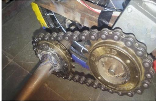
Figure 2. Chain Drive mechanism
