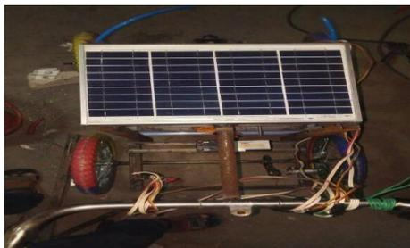
Figure 6. Power supply unit
