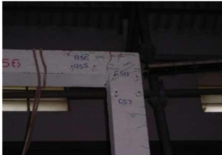
**Figure 4 Shear cracks in the front column**
