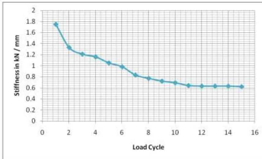
Figure 6 Stiffness of Test Specimen RCBF2
