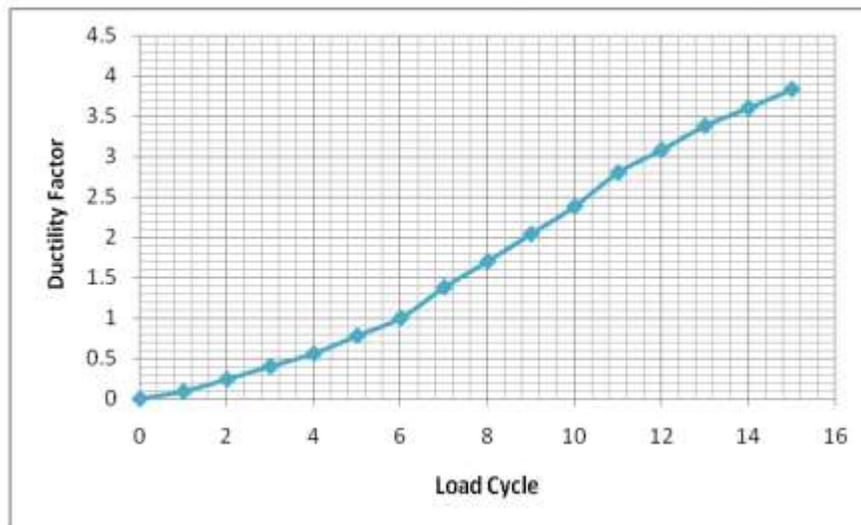
Figure 8 Ductility Factors for Frame RCBF2
