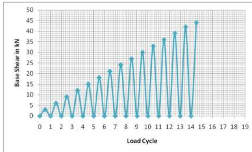
Figure 2 Sequence of Loading for the Frame RCBF 2
