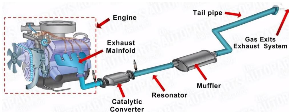
Fig.1 Position of Catalytic Converter
