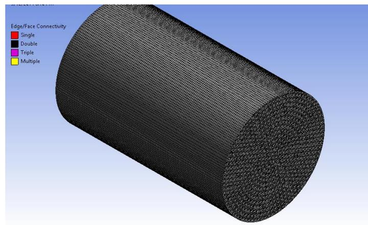
Figure 1 Modeling – CFD Catalytic converter
